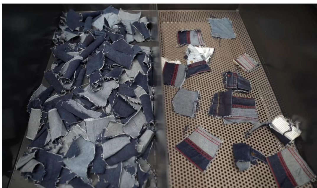
Figure 8 Clippings with trims (right) separated from untrimmed clippings (left) by Valvan's Trimclean™ technology ( https://www.valvan.com/en/solutions/textile-sorting-recycling )
